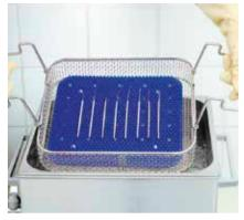
Cleaning of micro instruments in insert basket K 14. Free of contact on silicone knob mat SM 14.
