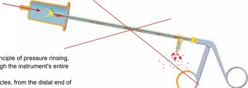
When cleaning according to the principle of pressure rinsing, all dirt particles are conveyed through the instrument's entire lumen.
